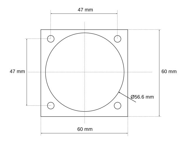
Mounting holes are provided with M3 thread and 4 mm thread depth.
