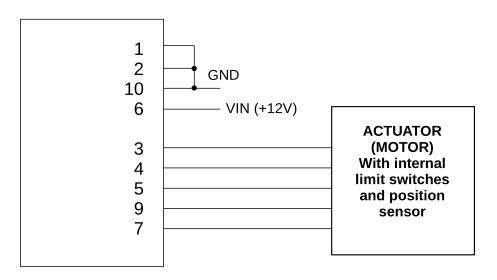
**ATTENTION!** Always refer to the documentation for the actuator used to identify the appropriate signals for the motor and position sensor. Then connect to the corresponding pins of the control unit connector, which are described in the table in chapter 4.4.
